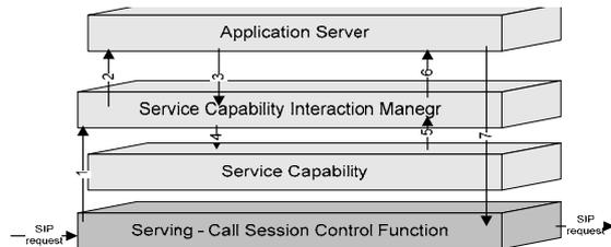
Figure 3: Proposed Service Composition Management Mechanism
