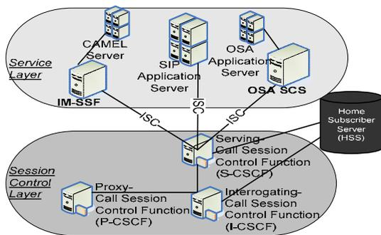
Figure 1: Functional Architecture of IMS
