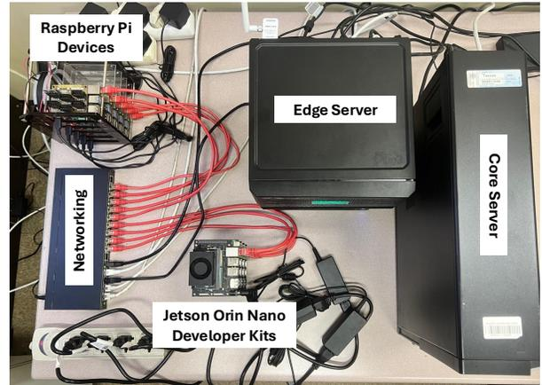
Fig. 4: Laboratory Setup for Edge and Core Deployment
