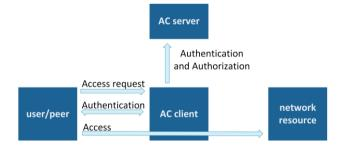
Fig. 1. Functions of AC systems.
