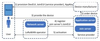
Fig. 4. LoRaWAN AC model with the first scenario of the OTA activation process. The device belongs to a specific service provider.
