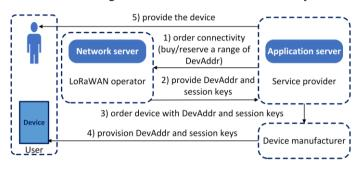
Fig. 6. LoRaWAN AC model with the ABP activation process.
