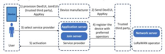
Fig. 5. LoRaWAN AC model with the second scenario of the OTA activation process. The device does not belong to a specific service provider and a user can buy it from any retail channel.
