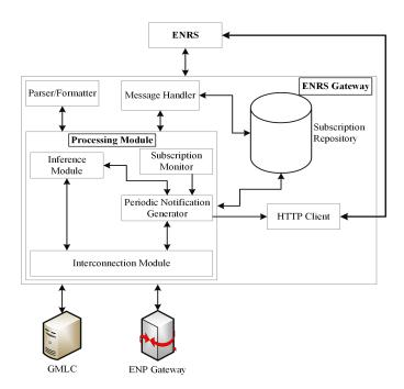
Fig. 2. ENRS Gateway architecture
