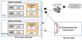
Fig. 3. Connection logic component initialization.
