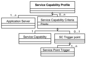
Figure 5: Proposed Service Capability Profile of Application Server
