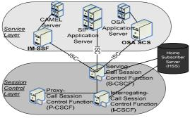
Figure 1: Functional Architecture of IMS
