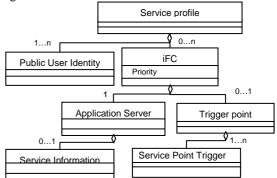
Figure 2: A Subset of IMS user Service Profile
