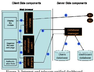
Figure 3: Internet and telecom unified dashboard Architecture
