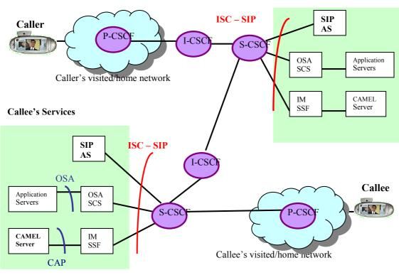
Figure 1: service architecture in the IMS
